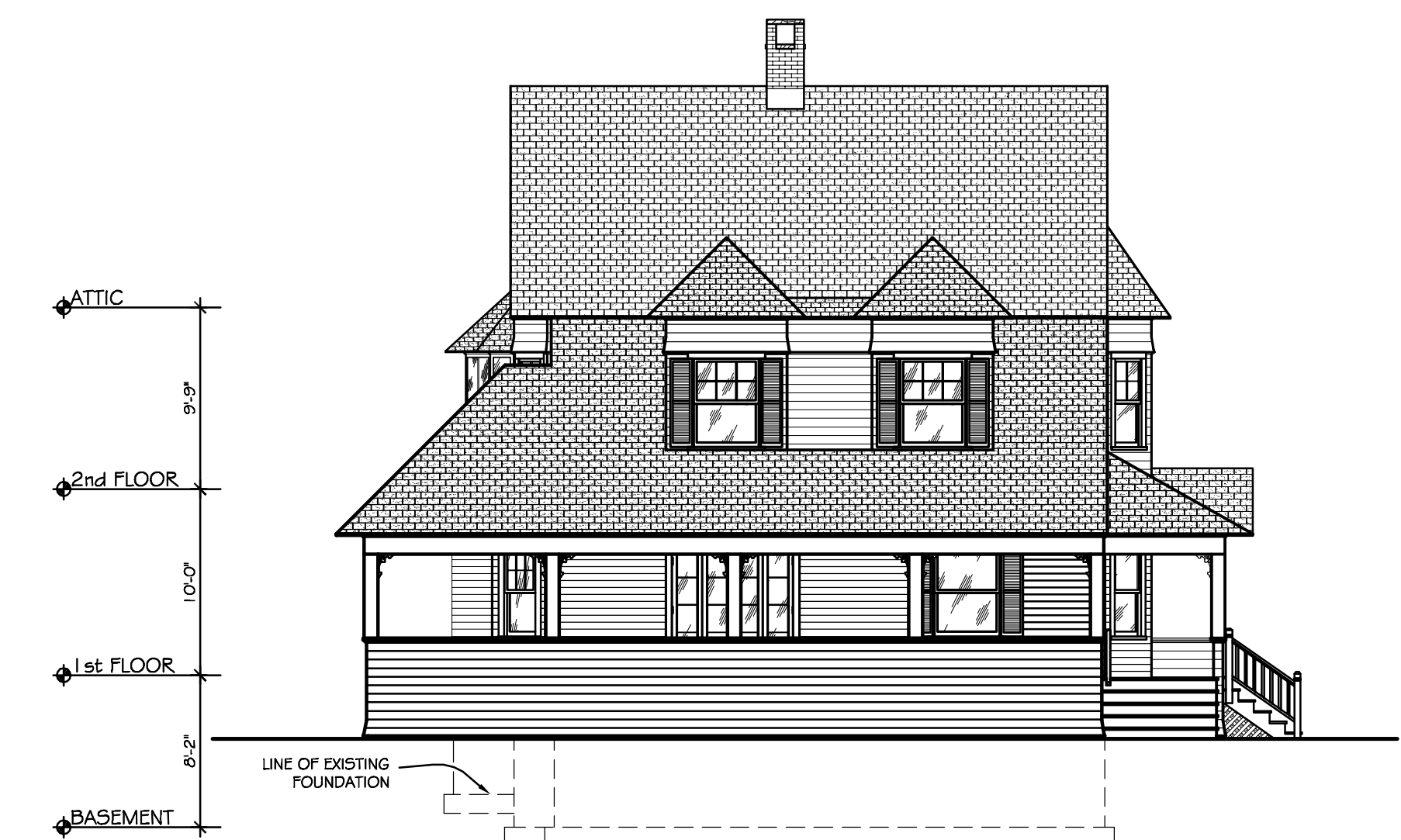
4 EXISTING EAST ELEVATION 1/8" = 1'-0"
