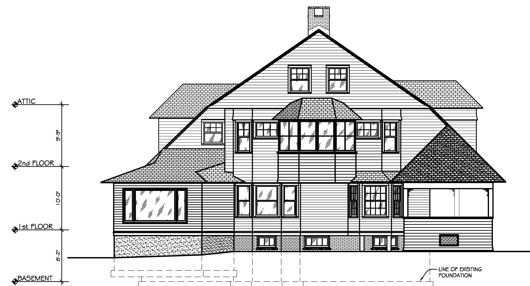
7 EXISTING SOUTH ELEVATION 1/8" = 1'-0"
